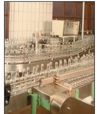
uni SS 812 & uni SS 881 TAB Straight running Bottle inspection
